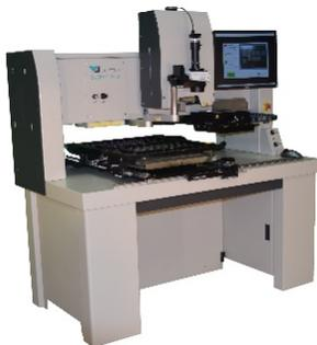
The Summit 1800i offers everything customers liked about the Summit 1800 plus more. The rework system provides the highest speed and accuracy for large boards (up to 560 x 762mm). Now available with 80mm component alignment capability, the 1800i is the leading choice for DIMM connectors and CPU sockets.
